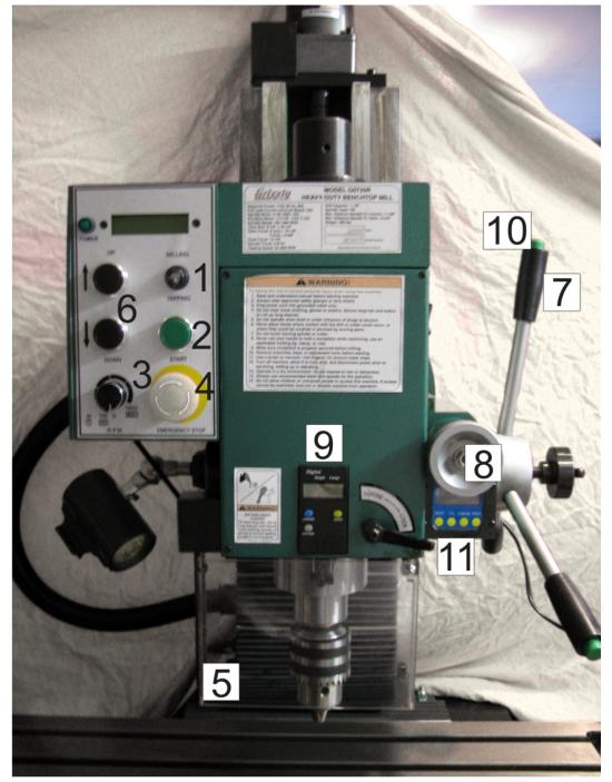
**Fig.:** Front side of the mill. (1) milling/tapping selection; (2) start; (3) RPM; (4) emergency off; (5) chip guard; (6) column up/down; (7) spindle feed; (8) spindle fine feed; (9) column "DRO"; (10) reverse spindle rotation; (11) digital protractor
